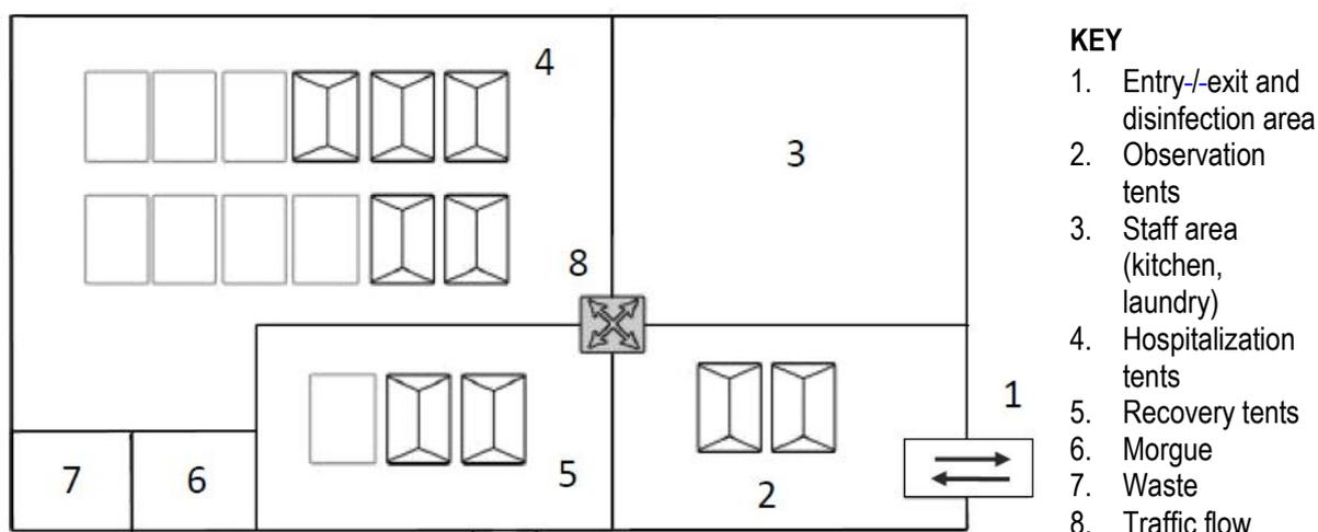
**Fig. 1. Example of CTC (schematic)**
